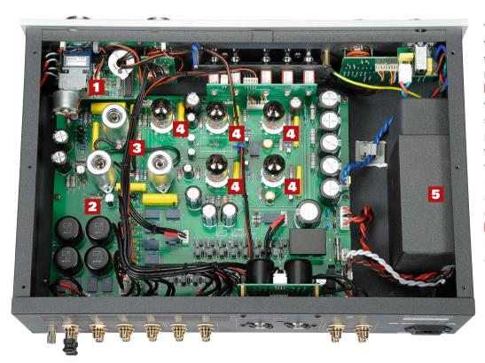
The volume control in the preamplifier is done traditionally via a, here, motor-driven potentiometer . In the Phono-MC stage, two pairs of transformers switchable from the front panel 2 raise the currents for the following tubes 3, which are shielded against interference. The main amplifier consists of five double triodes of type ECC82 4. The mains transformer 5 is encapsulated to protect against interference.
