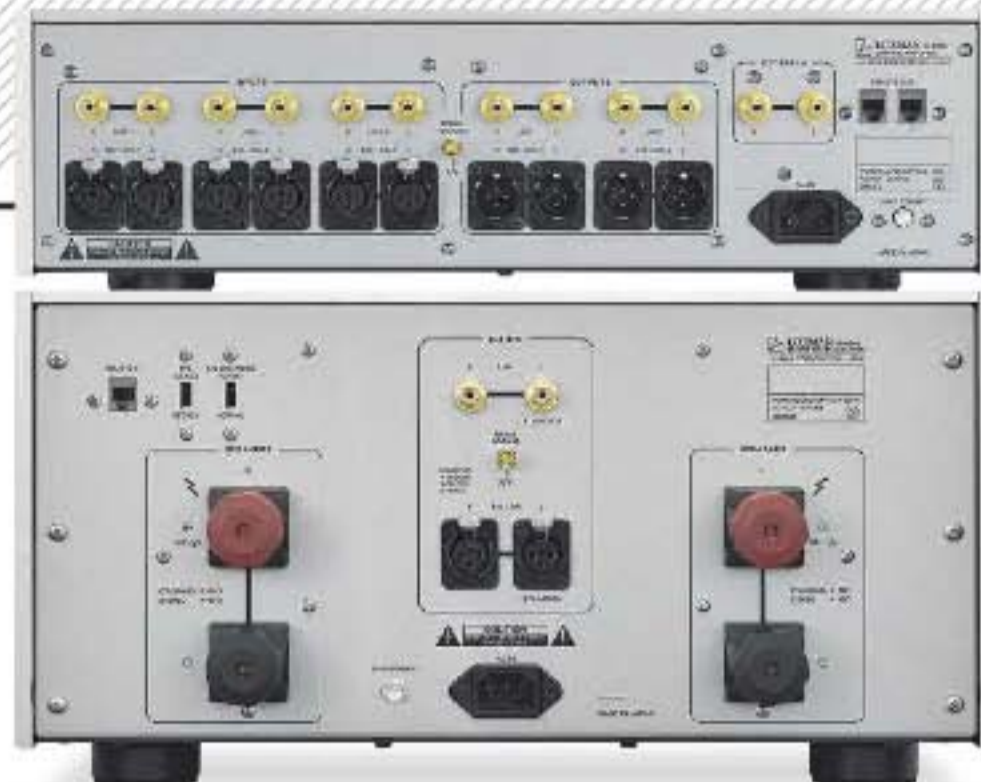
ABOVE: The preamp (top) offers six line inputs (three on RCA, three balanced on XLR) together with an external preamp input, and four line outputs (two each on RCA and XLR). The power amp (below) has huge 4mm speaker posts plus balanced and single-ended (RCA) inputs. The M-900u can be bridged as a mono amplifier
